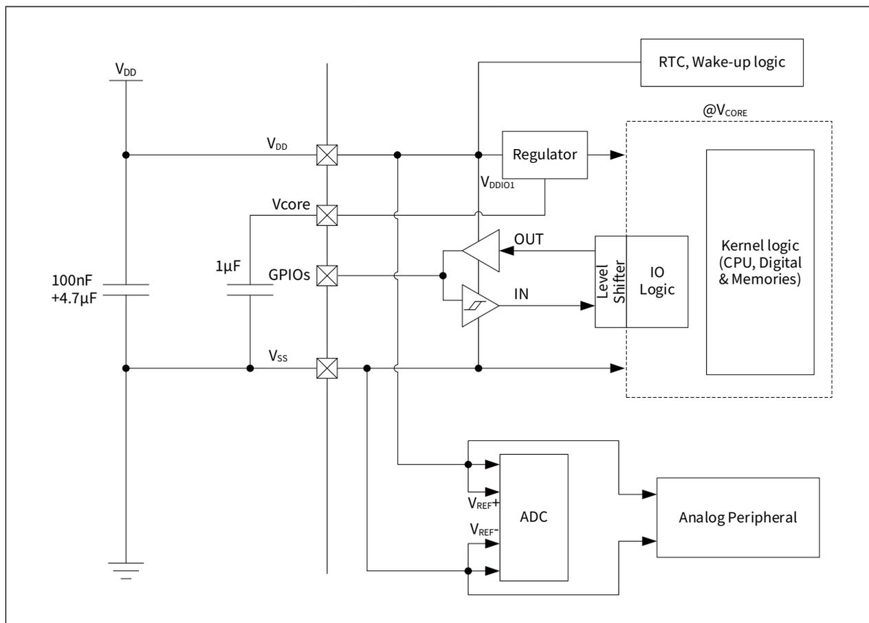
*Caution 1: Each power supply pair ( $V_{DD}/V_{SS}$ ) must be decoupled with filtering ceramic capacitors as shown above. These capacitors must be placed as close as possible to, or below, the appropriate pins on the underside of the PCB to ensure the good functionality of the device.*
