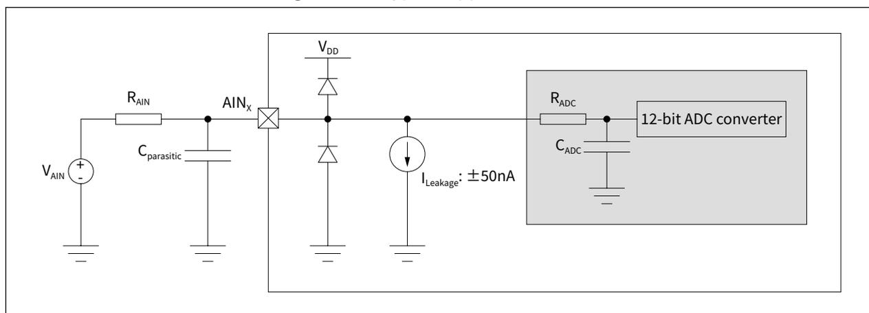
The following formula is used to calculate the maximum value of the external input impedance so that the sampling error can be less than 0.5 LSB:
