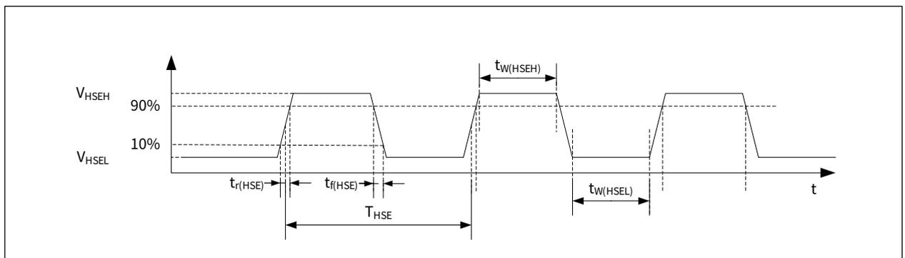
**Low-speed external user clock generated from an external source**
