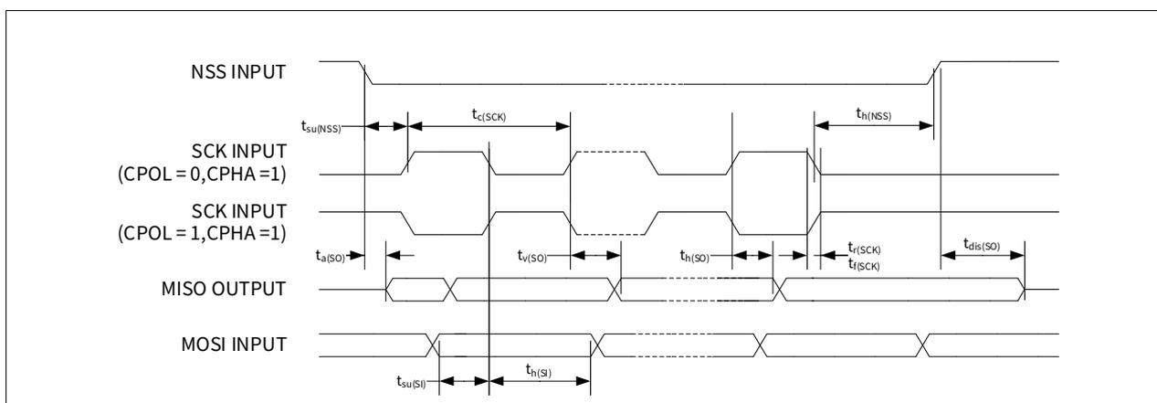
Figure 7-14 SPI timing diagram - master mode
