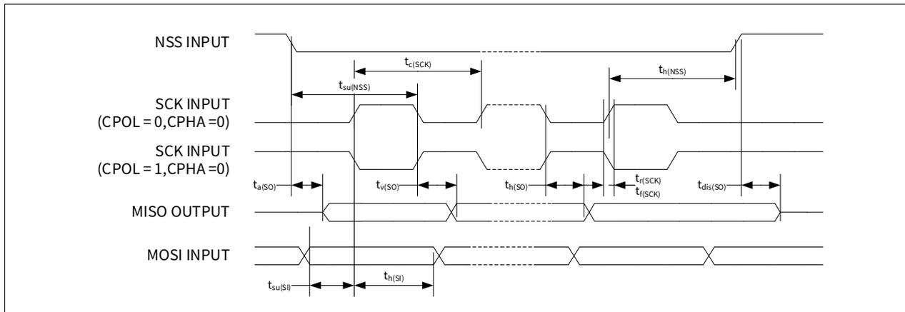
Figure 7-13 SPI timing diagram - slave mode and CPHA=1
