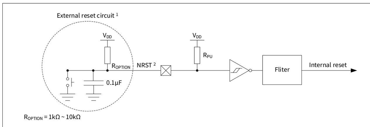
**Caution 1:** The external capacitor protects the device against parasitic resets.
